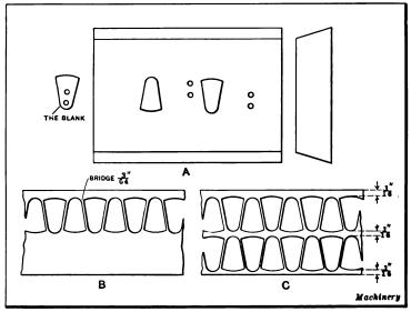
Fig. 4. Double Blanking and Piercing Die — Appearance of Stock that is passed through the Die
